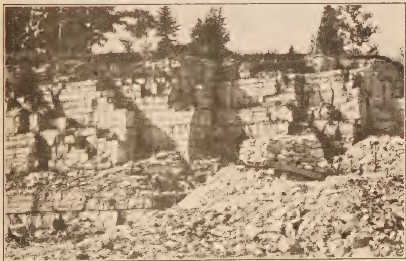
FIG. 1. — Niagara limestone, showing well-bedded layers with two sets of strong joints at right angles to each other. (U. S. Geol. Surv.)
